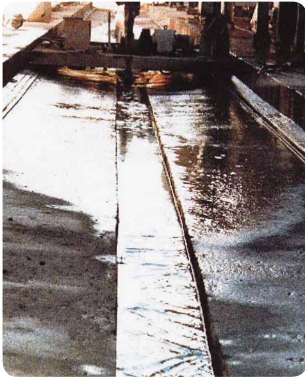
Photo 55. Channel for the conveyance of the waste sludge from a bandsaw
