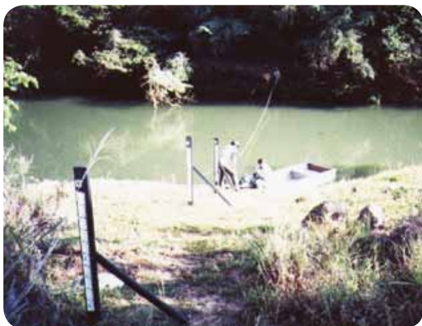
Photo 72. Water level rulers – Entre-Ribeiros stream
