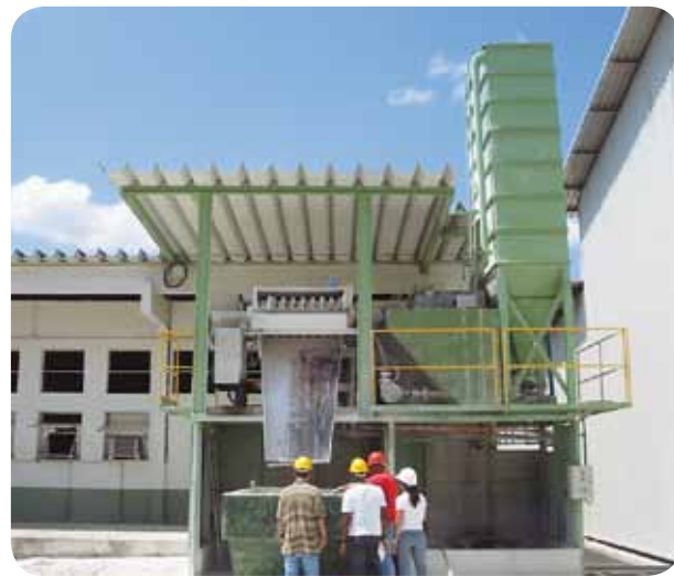
Photo 67. The filter-press
