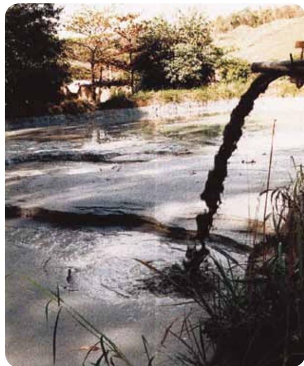
Photo 57. A typical tank for final disposal of the waste from the sawing of ornamental rock blocks (disposal)
