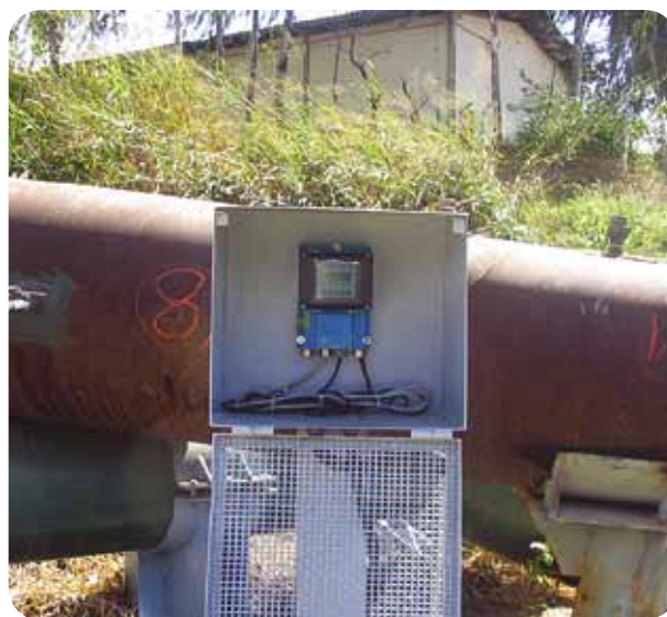
Photo 74. Flow Meter – Thirty-foot pipe
