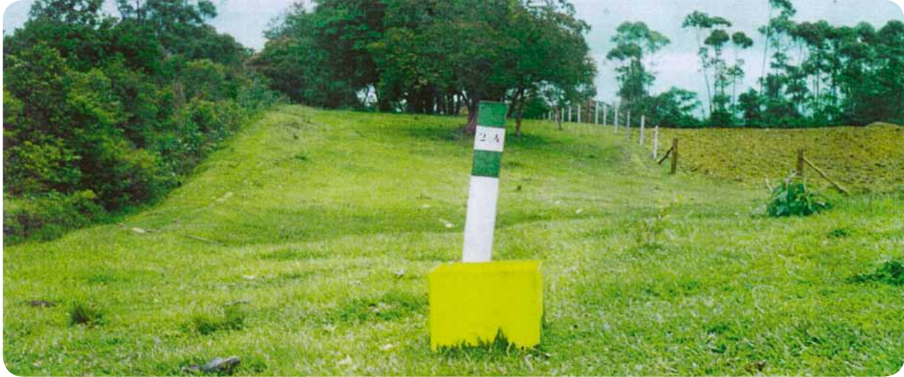
Photo 49: Piezometers
